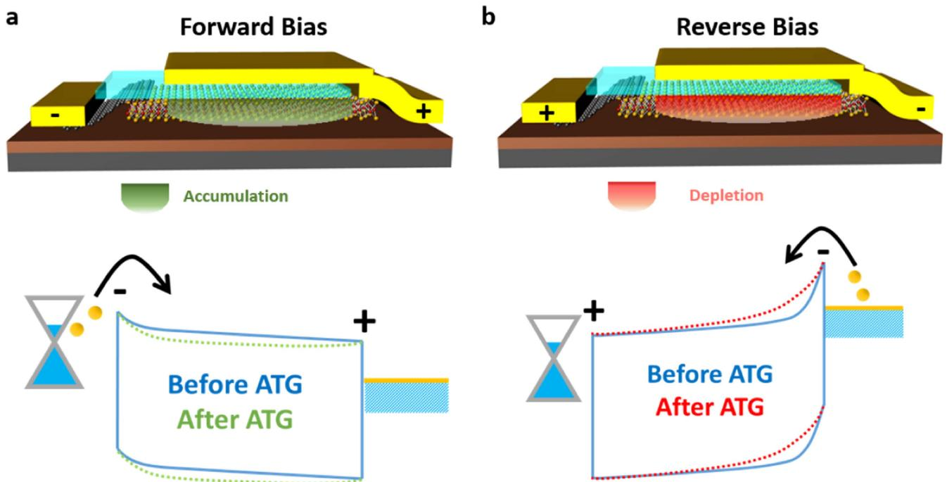
**Figure 2.** (a) Schematic and band diagram showing contacts polarity and electron accumulation in MoS<sub>2</sub> during forward bias, (b) schematic and band diagram showing contacts polarity and electron depletion in MoS<sub>2</sub> during reverse bias.
