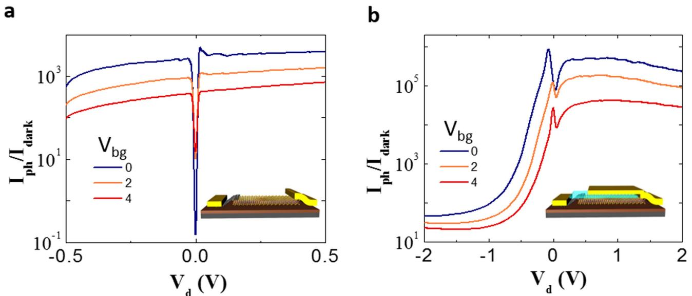
**Figure 4.** Plot of relative photo current and drain voltage of GM device, (a) before the deposition of ATG (b) after the deposition of ATG.
