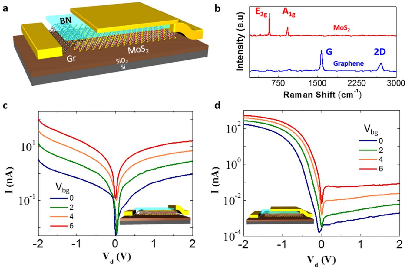
**Figure 1.** (a) Schematic of the GM self-gating diode, (b) Raman spectra of MoS<sub>2</sub> and graphene, (c) output characteristics of GM diode before the incorporation of ATG (semi-logarithmic scale), (d) output characteristics of GM diode after the deposition of ATG (semi-logarithmic scale).
