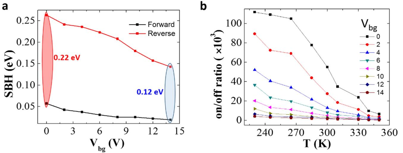
**Figure 3.** (a) Effective SBH obtained from temperature dependent measurement at different back gate voltages during forward and reverse bias, (b) plot between rectification ratio of device and temperature at different back gate voltages.
